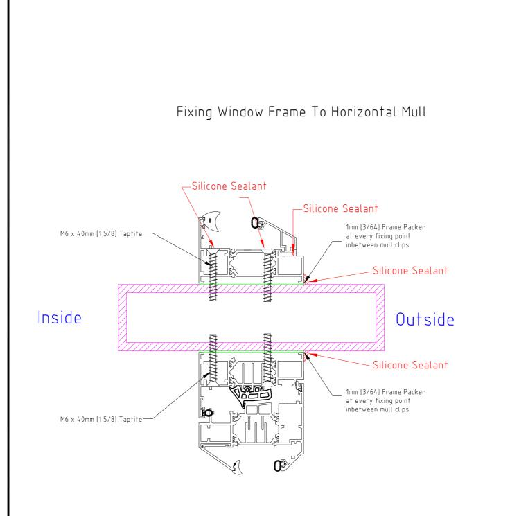
SEALANT TO BE APPLIED ON SITE BY INSTALLER.
