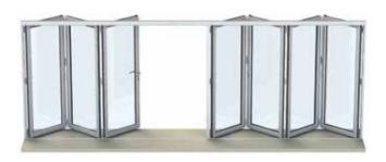
Ideal for larger openings, the 3+3 is one of the most diverse configurations as it can operate as a French door at the center, have 3 doors opening one way while the other 3 remain closed, or they can be opened fully with 3 doors folding each way to offer complete symmetry.
